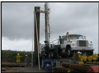
Exploratory drilling for geothermal energy on Nevis
